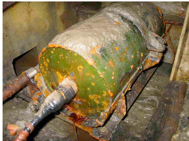
The small swimmer delivery vehicle (SDV) found within the ILC is similar in construction and dimensions to previously captured SDVs. It is approximately 1.7 meters long, .3 meters in diameter and has a .4 meter diameter caged prop. Handles for swimmers and attachment points for equipment are welded to the SDV.
