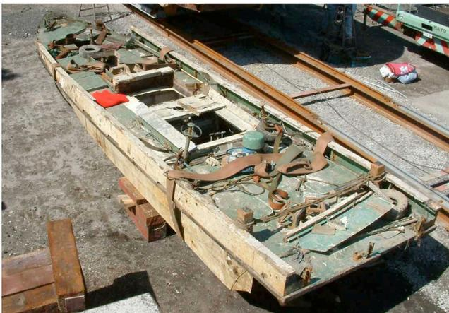
The ILC craft found aboard the salvaged vessel is based upon an older design that has been frequently encountered during operations against the Republic of Korea (ROK). It has an overall length of 11 meters and a maximum width of 3 meters. It is constructed with five main compartments (engine, steering, passenger, main cargo and forward cargo). Stored within the main cargo
