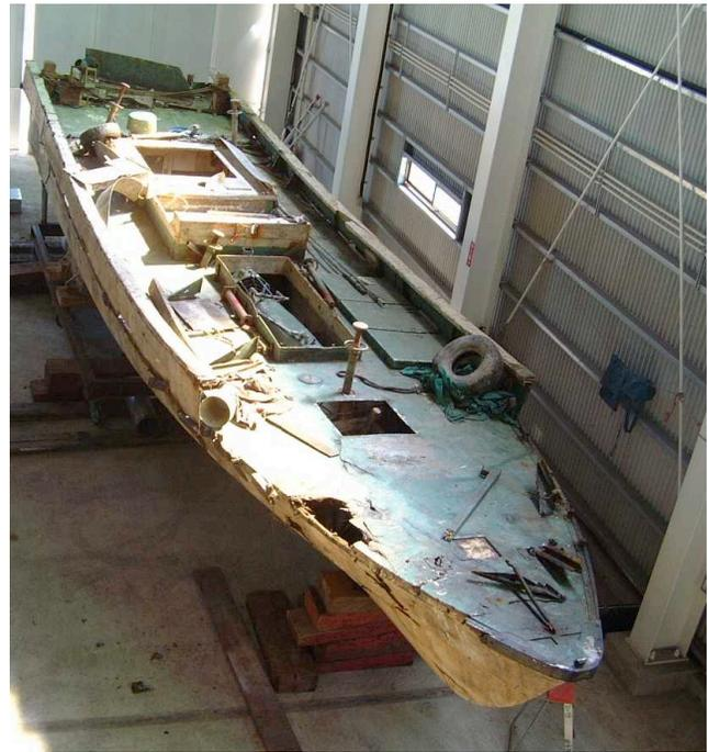
was a small swimmer delivery vehicle. The deckhouse is constructed of wood and the hull is coated with fiber resin plastic. The steering compartment has a single wheel and three throttle levers to control the three high-speed marine engines and basic instrumentation. The ILC also mounted a small 20 cm by 30 cm cylindrical explosive charge to be employed to kill the crew and prevent the capture of the craft.
